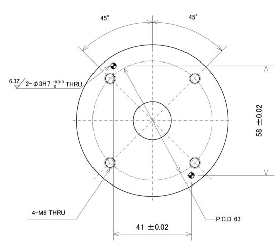
According to the diagram above, open mounting holes for the robot from the force sensor mounting side.
